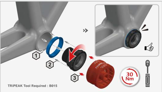
If the non-drive side BB rotates along with the drive-side BB during installation, prepare another BB wrench (B015) to secure the non-drive side BB in place, ensuring the required torque value is reached.
